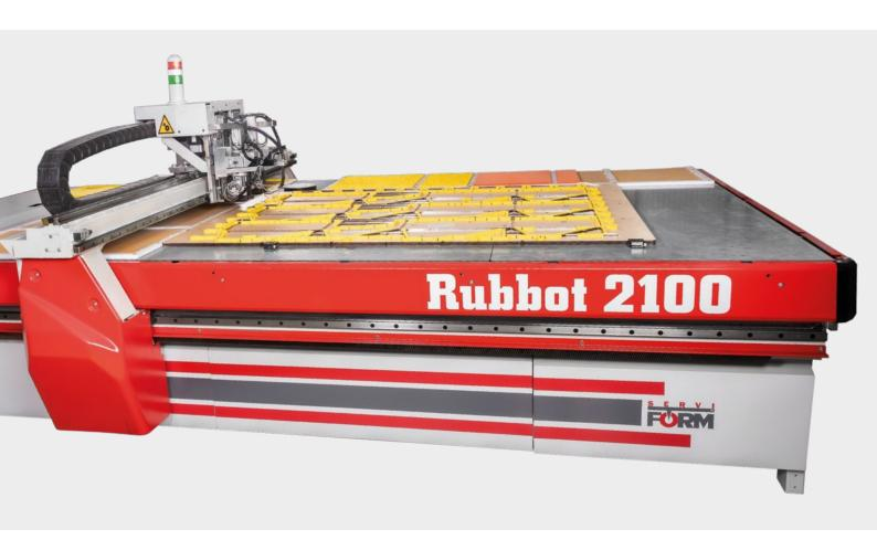
The fully automatic robot for installing ejection rubber on flat dies.
