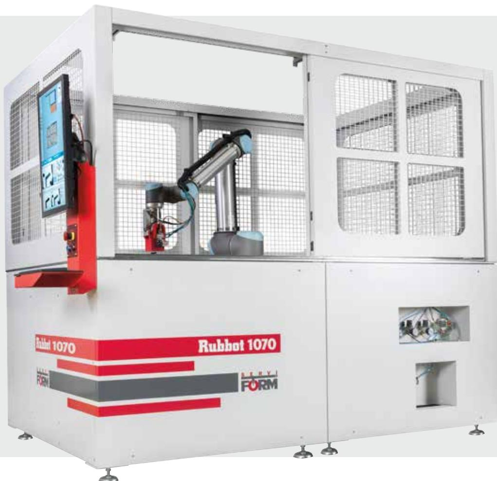
A fully automatic robot for installing ejection rubber on the die!
