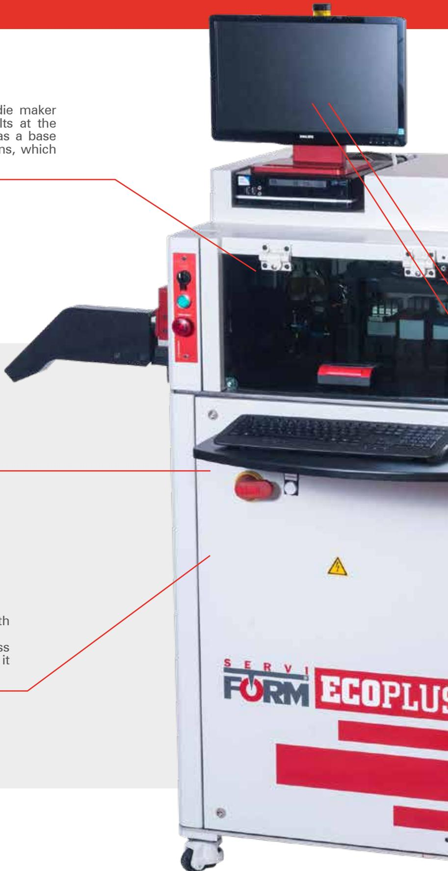
All special options such as perf, cut crease, dove tail, broaching and nicking, just to name a few, are available with the initial purchase or at any time in the future. Four nicks per second are produced using a 4 position Revolver Nicking cartridge, while ensuring burr free placement accuracy with a lower tool bevel support.
